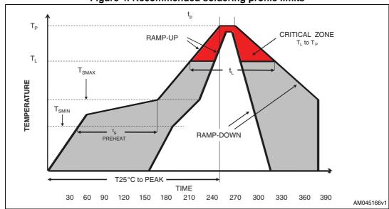
Figure 4. Recommended soldering profile limits
