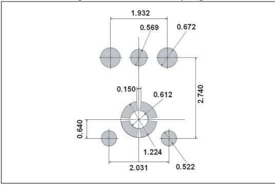
Figure 7. Recommended stencil openings
